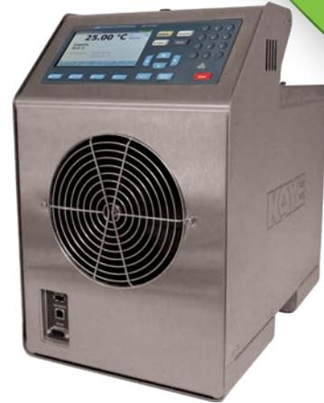
The Kaye CTR-25 is the latest addition to our complete line of advanced calibration dry blocks and baths designed to address the specific needs of thermal Validation.
